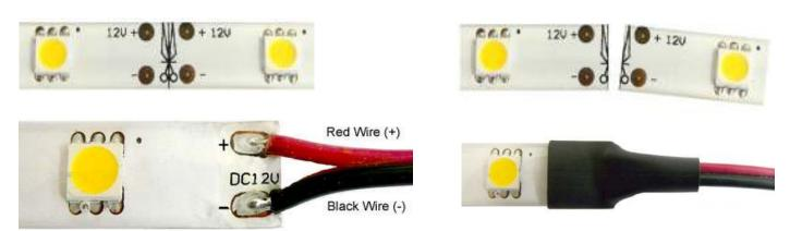
You need to cut the Strip along the line with the 4 solder pads on either side of the cut.
